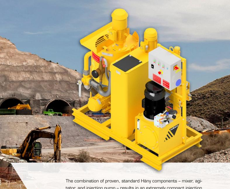
The combination of proven, standard Häny components – mixer, agitator, and injection pump – results in an extremely compact injection plant. This setup is suitable for a wide variety of applications such as anchor, sleeve pipe, and contact injections.
