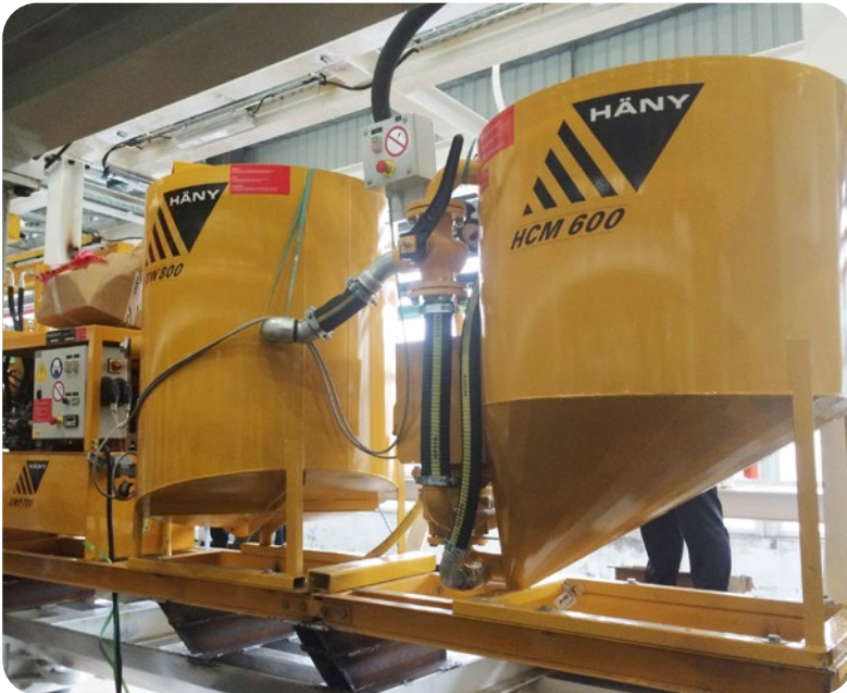
Häny Grout Plant IC 1400/725 installed on the backup of the TBM from China Railway Engineering Equipment Group (CREEG)
