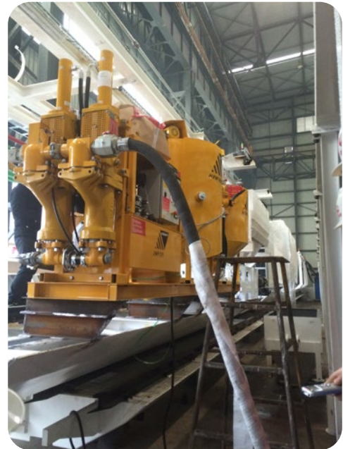
Häny Grout Plant IC 1400/725 installed on the backup of the TBM from China Railway Engineering Equipment Group (CREEG)
